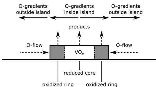
**Fig. 4.** Schematic drawing explaining the existence of oxygen gradients inside and around  $\text{VO}_x$  islands supported on  $\text{Rh}(1\ 1\ 1)$  during catalytic methanol oxidation. For details please refer to the text.
