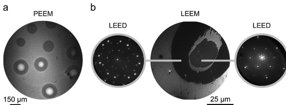
**Fig. 2.** Substructure of circular  $\text{VO}_x$  islands under reaction conditions, as demonstrated by PEEM and LEEM images. a) PEEM image recorded at 1030 K in an atmosphere of  $3 \cdot 10^{-4}$  mbar  $\text{CH}_3\text{OH}$  and  $1 \cdot 10^{-4}$  mbar  $\text{O}_2$ . b) LEEM image recorded at 2 eV and corresponding LEED patterns acquired at 50 (left) and 65 eV (right) in  $1 \cdot 10^{-4}$  mbar  $\text{CH}_3\text{OH}$  and  $1 \cdot 10^{-4}$  mbar  $\text{O}_2$  at 1030 K.
