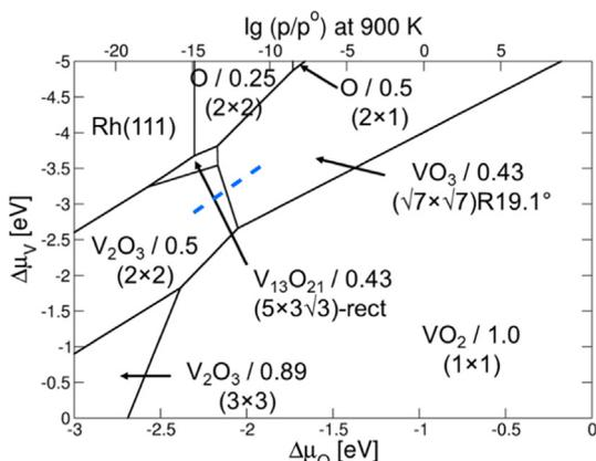
**Fig. 5.** DFT phase diagram of 2D  $\text{VO}_x$  phases with a coverage of  $\theta_V \leq 1\ \text{MLE}$ . The chemical potential of oxygen has been translated into a pressure scale based on tabulated data for 900 K. The V coverages in MLE as well as the surface structure are given with the composition of the corresponding oxide phase. The dashed blue line indicates a possible phase transition during the island oscillations described in the text.
