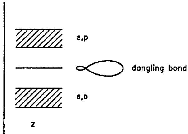
Figure 2.35. Shockley surface state or dangling bond in the almost ideal hybridization limit.
