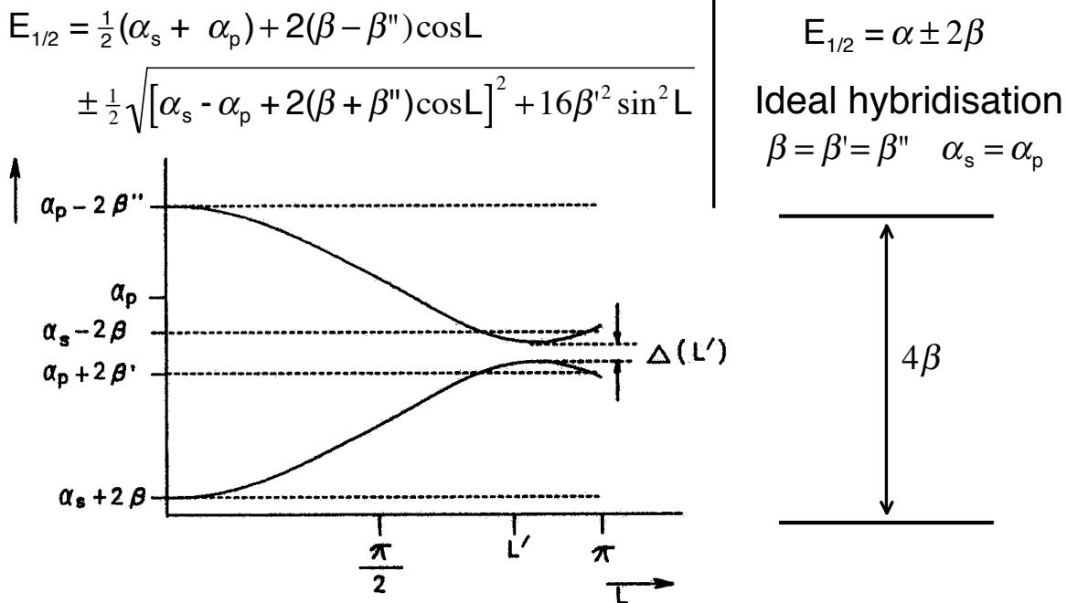
**Figure 2.34.** Overlapping crossing s- and p-atomic valence electron bands.
