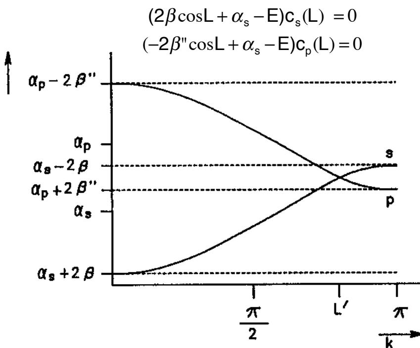
Figure 2.33. Overlapping non interacting  $s$  and  $p$  atomic valence electron bands –
